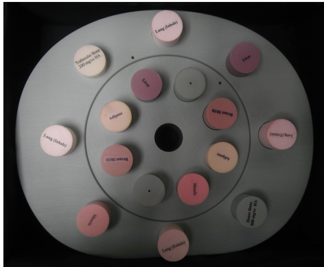
Figure 1: CIRS 62 electron density phantom, pictured with included tissue-equivalent inserts placed in bores. The inner “head” portion can be removed or it can remain in place to simulate a “body” measurement.
