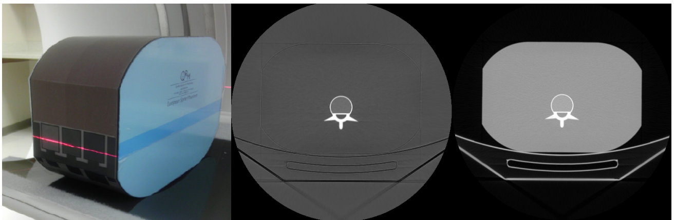
Figure 53: Left: The European Spine Phantom. Center: DECT K_2HPO_4 material density map. Right: SECT 80 kVp HU image.
